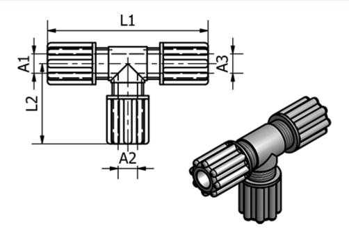
Ext. Hose Diameter A1 = 4/6Ext. Hose Diameter A2 = 4/6Ext. Hose Diameter A3 = 4/6L1 = 25L2 = 25
